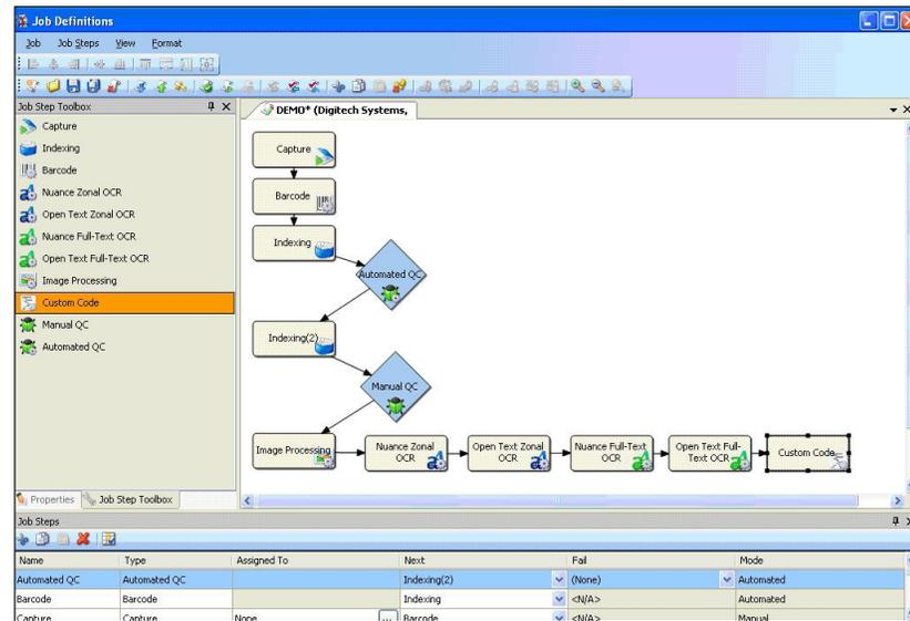
In PaperVision Capture, job workflows can be constructed via an intuitive drag-and-drop flowchart designer.
